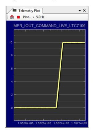
e. If you want to change the IDAC current to a negative value (meaning sinking current), you need to change the MFR\_IOUT\_MAX\_LTC7106 to a negative value first (see data sheet for more details).
