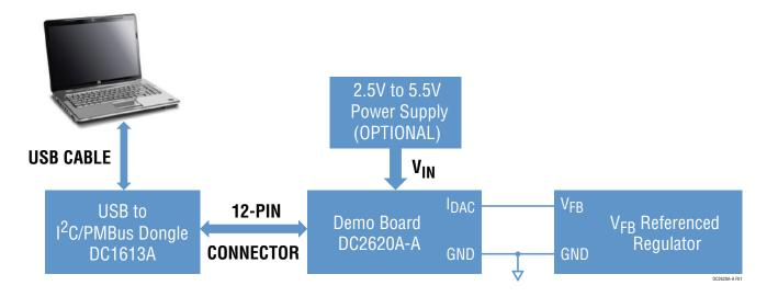
Figure 1. Demo Setup with PC
