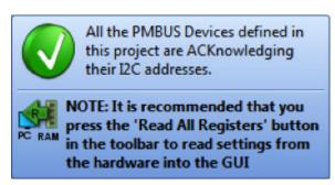
c. In the Toolbar, click the "R" icon PC) to read the RAM from the LTC7106. This reads the configuration from the RAM of LTC7106 and loads it into the GUI. When first powering on, you should read IDAC current at zero (high impedance IDAC) due to the LTC7106's internal power-on reset circuitry until a valid write takes place. The IDAC current value can be plotted in real time, shown in the following screenshot (at zero when first powering on):
