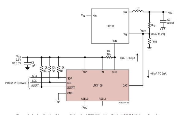
Figure 2. An Application Diagram Using the LTC7106 with a Typical DC/DC Voltage Regulator
